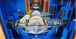
**In 2022** - GEMWELL successfully developed the "3500RPM serve spit tape constant tension taping machine". Compared with various taping machines in the wire industry, it has subversive design concept and formed a competitive advantage in terms of productivity and quality stability. One machine is equivalent to two machines, easy operation, quality stable. It is the preferred model for high-end signal cable.
