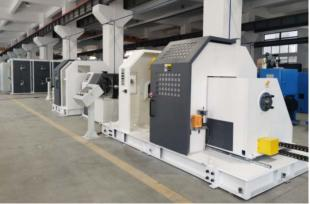
**In 2013** - GEMWELL has successfully developed "3000RPM constant tension copper wire bunching machine" and "alloy conductor backtwisting machine" with stable pitch. After backtwisting, there is no internal stress inside conductor. The production capacity is more than 5 times that of the tubular stranding machine and cage stranding machine.
