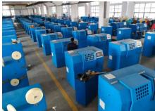
**In 2017** - GEMWELL successfully developed the "three core twisted pair taping machine". The signal cores pair twisted and tape wrapping are processed at one time to reduce the process flow and backtwist 100%. The twisted products have no internal stress and improve the cable structure stability.
