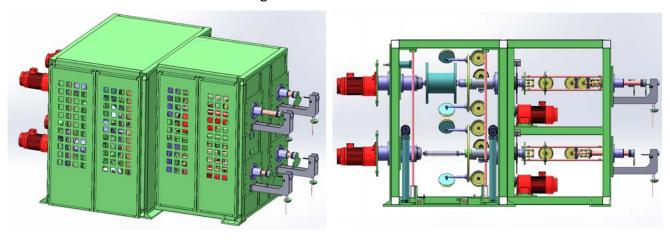
In **2021** - GEMWELL successfully developed the "rotary capstan". Equip with central rotary backtwist payoff and large cantilever single twist strander, it has solved the problem of high speed cabling for large cables OD more than 30mm. The cabling speed is about 5 times that of the traditional cage strander.
