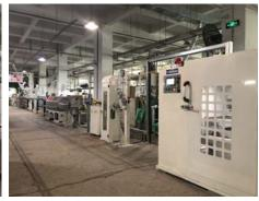
**In 2015** - GEMWELL has successfully developed "65 high speed continuous drawing & annealing & extrusion tandem insulation line" with line speed up to 1500m/min, cable each performance all excellent.
